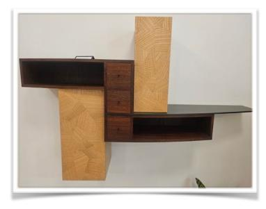
• Cracked ice pattern of veneer - laser cut individual pieces - edges were burned by the lazer so he used a hand file to shave off the burnt edges (see picture)
