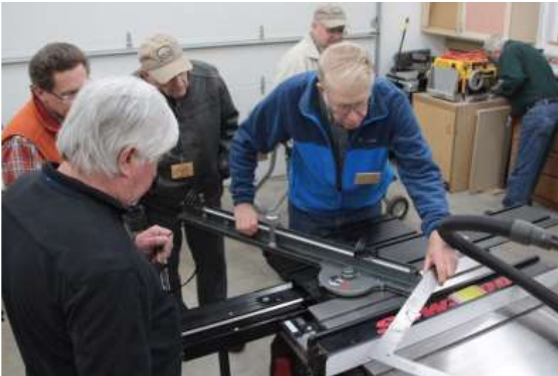
Dick Schofield's shop has a nice sled attachment to his Saw Stop
