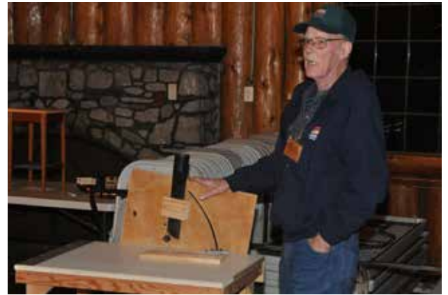
Bill Baer , showing a jig he made for using a router in the horizontal position to make cabinet door panels.
