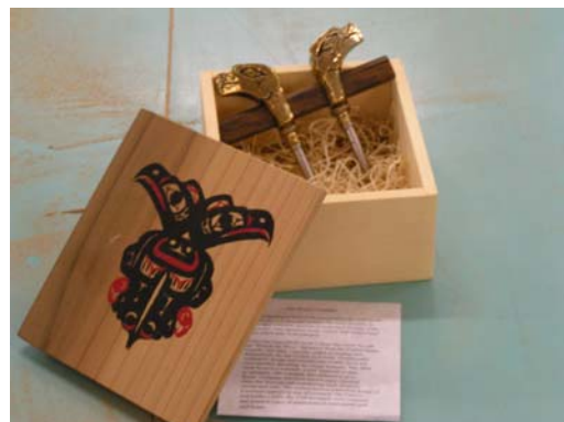
A door prize won by Vern Tator at an antique tool collectors banquet. The trammel points were cast in a numberd series. The box is steam bent cedar with a native emblem.
