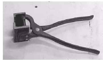
Left a Formica trimming "guillotine". Right a pair of scribes Vern uses to transfer profiles.
