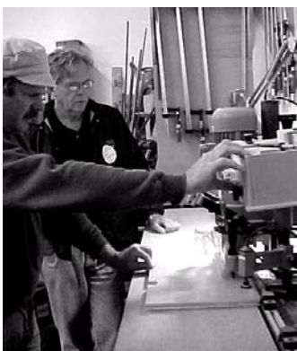
Gary demonstrating a machine used to drill multiple holes for shelf pins.
