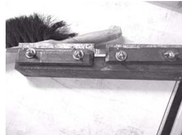
Band saw blade soldering clamp by Jim Murphy
