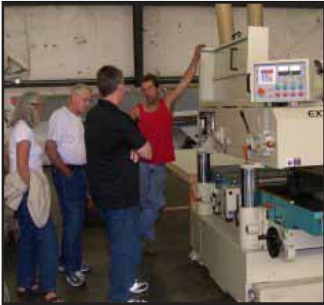
An Edensaw employee explains the workings of their new double sided planer to Val & Laura.....a finished board in one pass!
