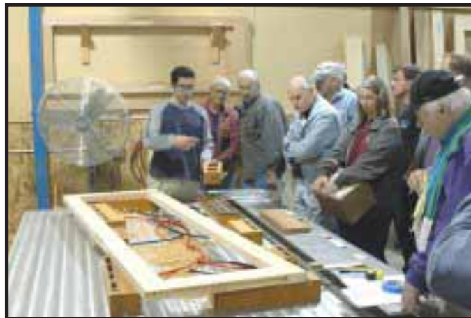
Orion explains & demonstrates how a door is set up on NorthStar Woodworks CNC router for final sizing and machining for hardware.
