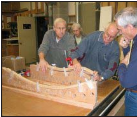
Cec demonstrated his jigs and techniques used in bending parts for his rocking chair.
