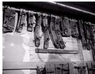
Left: Some of the many jigs used to shape profiles for various chair parts. Right: A two headed profile shaper.
