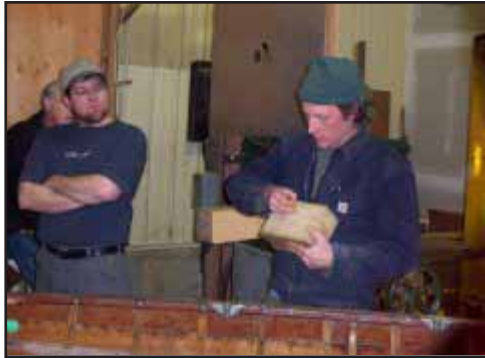
Andy Stewart and James McMullen demonstrating how to caulk between lapstrakes
