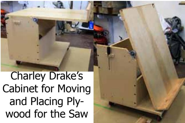
Charley Drake's Cabinet for Moving and Placing Plywood for the Saw
