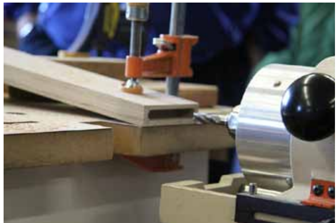
Horizontal Mortise at a 7 degree Compound Angle, as Demonstrated by Tom Dolese
