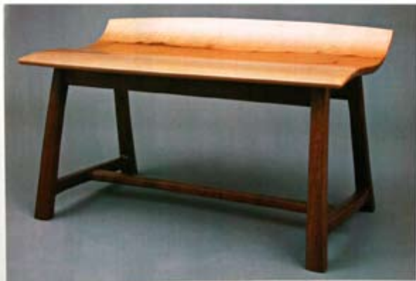
Bench by Greg Klassen, featured in Fine Woodworking. Coopered, then shaped with two wooden planes Greg made just for this project.
