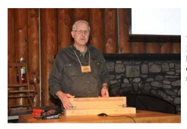
Val Matthews gave us another shop tool to make. His easily-made dovetail vice consists of some heavy wooden members and two sacrificial pipe clamps to give the fixture a great platform for routing both pins and tails
